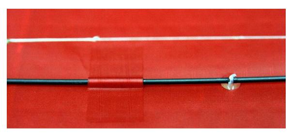
Photo 5 also shows how I attach the bridle to the frame, as seen from the rear of the sail.
